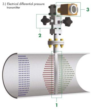
In the downstream chamber in the shadow of the sensor and thus partially shielded from the impact of flowing medium, negative pressure forms.
