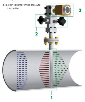
In the downstream chamber in the shadow of the sensor and thus partially shielded from the impact of flowing medium, negative pressure forms.
